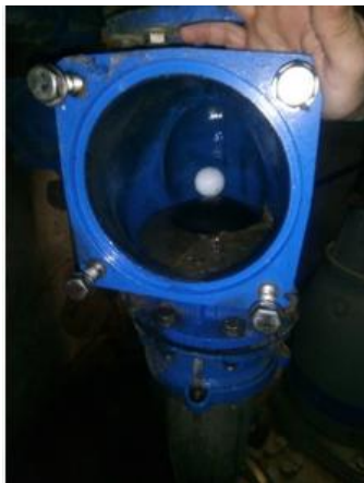
Figure 3 and 4: The ApoleAU In-Line Leak and Pressure Inspection Tool being inserted and extracted into wastewater pipeline3
