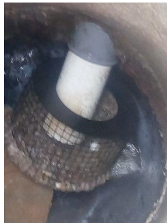
Figure 3 and 4: The ApoleAU In-Line Leak and Pressure Inspection Tool being inserted and extracted into wastewater pipeline3
