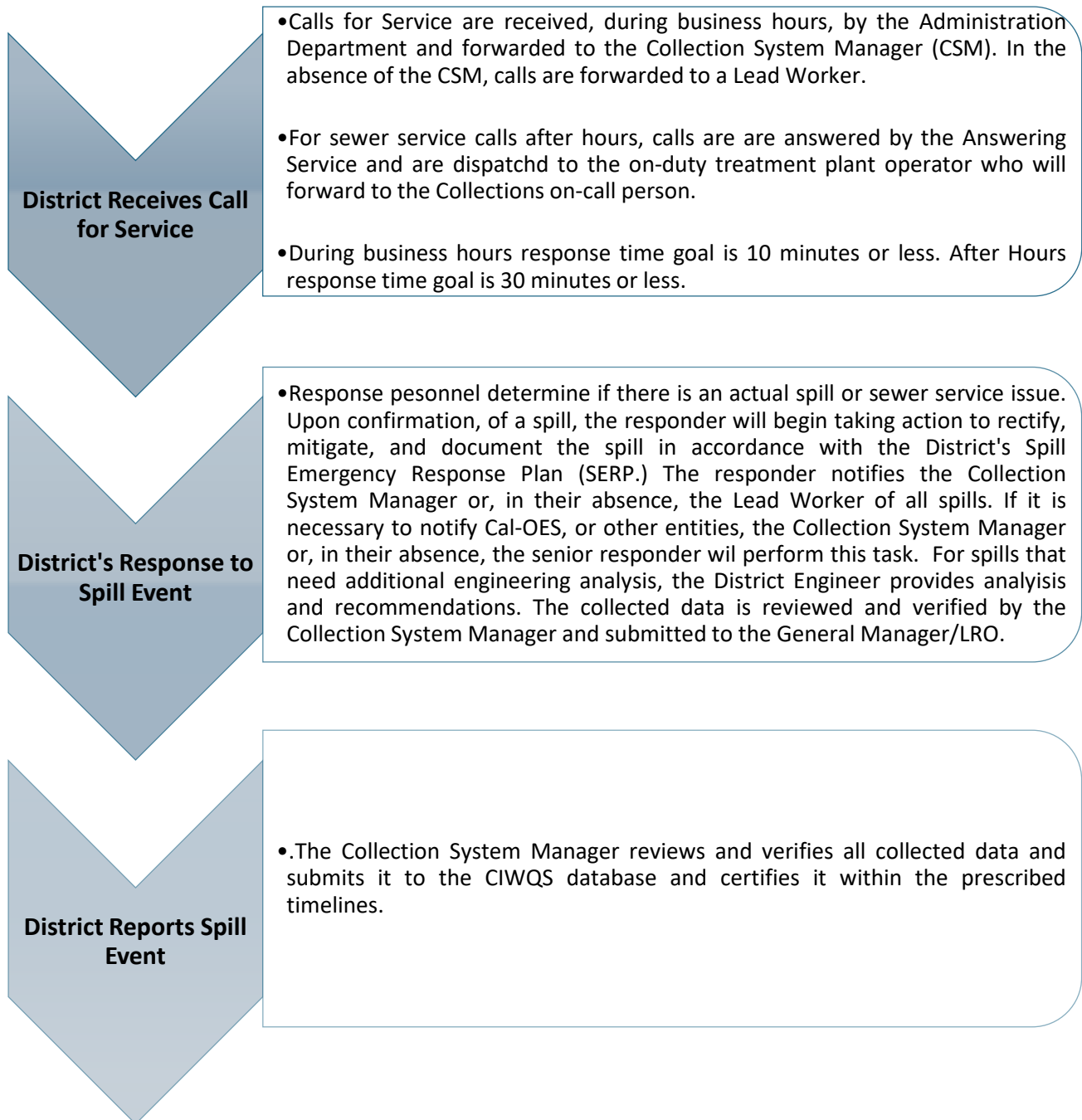
[Figure 6 - Chain of Communication for Reporting Spills]
